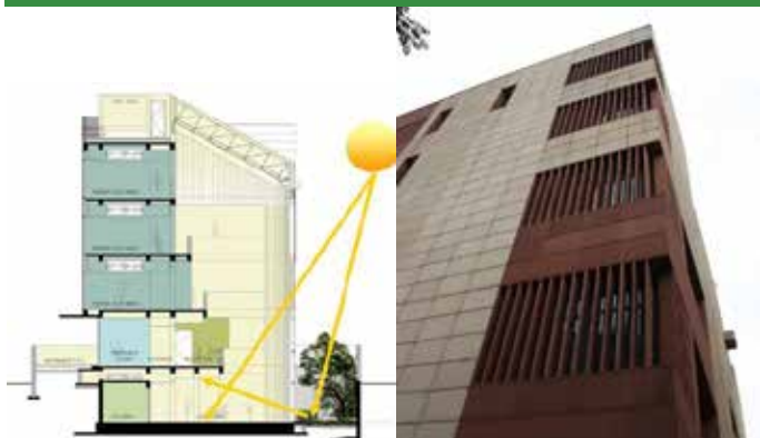
FIGURE 1: ENERGY EFFICIENT LIGHTING: MODELED DAYLIGHTING STRATEGY OF BASEMENT AND LEGACY SPECTRAL BUILDING'S RECESSED WINDOWS
